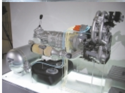
The Mazda gasoline/hydrogen RX-8 employs an electrically assisted turbocharger and electric propulsion motor.
