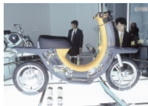
Yamaha's scooter fuel cell is a direct-methanol type.
