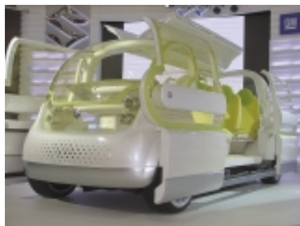
Suzuki's Mobile Terrace is based on GM's Hy-wire skateboard platform.
